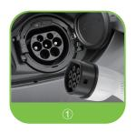
① Unlock the vehicle, press the power plug button on the vehicle side, and pull it out from the vehicle side base.
